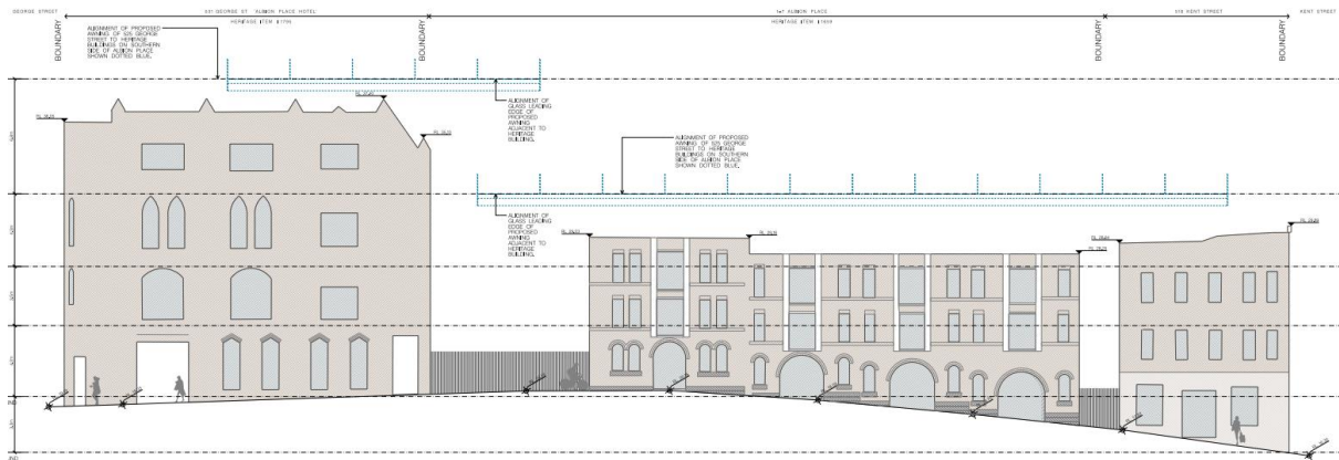
Figure 39: Albion Place south elevation showing alignment of the proposed awning in relation to adjoining buildings on opposite side of Albion Place
